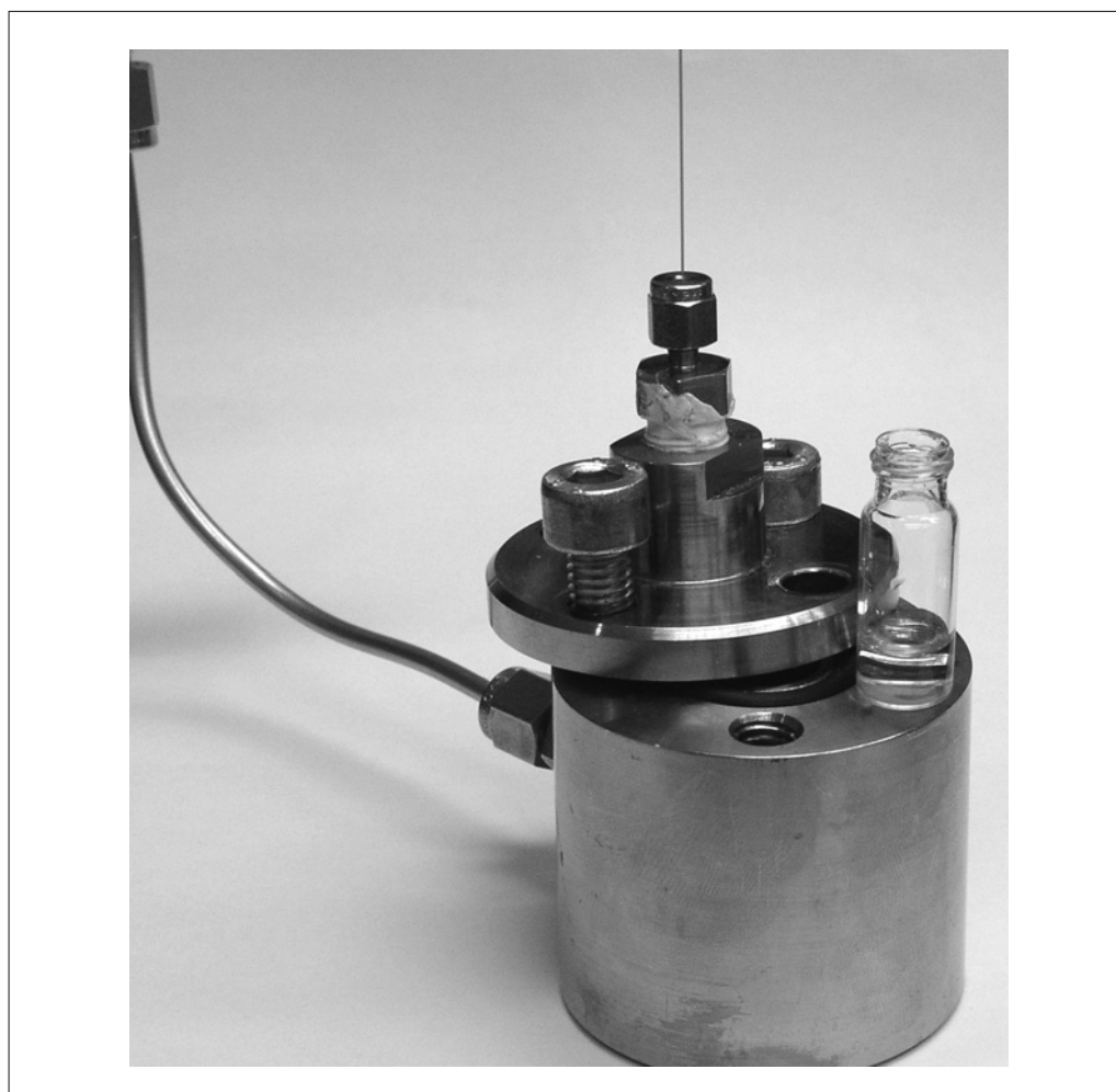
Figure 18.13.2 A pressure bomb used for packing resins and loading samples.
